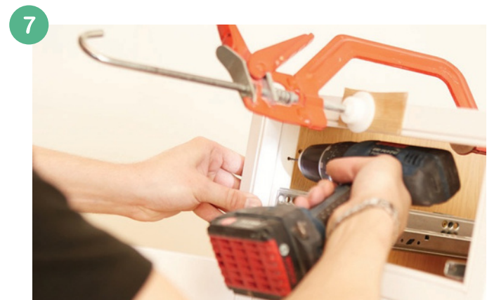
7 Pilot hole through the predefined holes in the fixing bars into the carcass.
